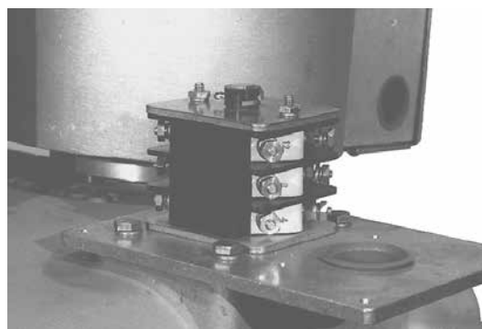
Figure 18. Auxiliary switch (with cover removed).
